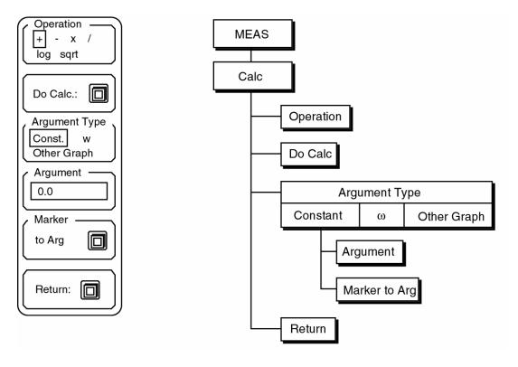
OperationThe Operation function selects the type of operation to be performed. The<br/>add, subtract, multiply, and divide functions require a second argument<br/>which may be a number, w (2πf), or the other trace. The log (base 10) and<br/>square root function require no argument.Do CalcPressing this key starts the actual calculation. The "Calculating" message
