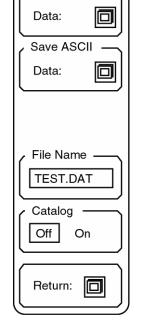
The first file will be highlighted and the file name will appear in the File Name field. Activating the cursor by pressing the [MARKER] key allows the knob to scroll through the directory. The highlighted file name will be copied into the File Name field. If the Save Data key is now pressed, the data will be saved under an existing file name and the previous version of that file will be lost. To create a new file name, use the File Name key.
