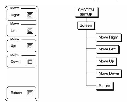
The screen position is stored in non-volatile memory and is retained when the power is turned off. To restore the screen to the default position, power the unit on with the [<-} (backspace) key pressed.
